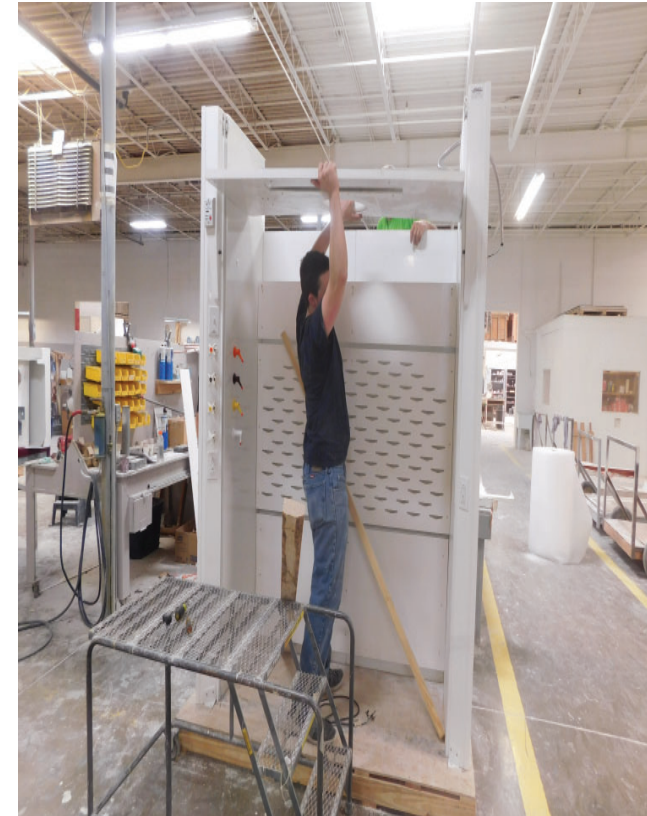
Set the rear of the Ceiling Panel on the flange at the top of the Rear Panel. Secure rear edge with provided.
