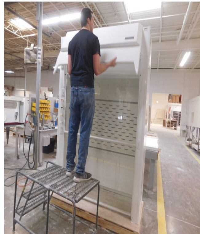
Install Front Access Panel.
