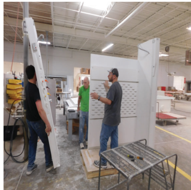
Set the Left Wall and Secure to Back Wall with provided #8 or #10 sheet metal screws. Utilized #8 screws first, however, due to pre-assembly the #8 screw may "strip" or may not "bite" then utilize the #10 screw. NOTE: Quick ratchet bar clamps to a stepladder may be used to partially support the components until other panels can be permanently secured.
